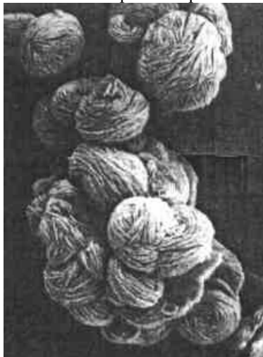
Fig. Coil morphology of Mo 4.6 O 12 NT
